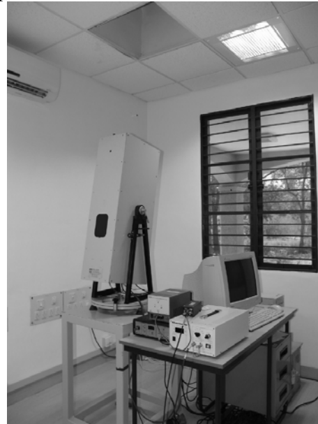
Fig.1 The portable laser radar system at NARL site
