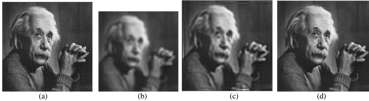
Fig. 3 The Great Scientist- Albert Einstein. (a) Original image, (b) Blurred, Noisy, Downsampled LR image [200 200], (c) Recovered Image with ringing with 100 iterations, (d) Recovered bicubic Interpolated SR image [800 800].
