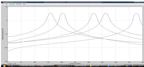
Fig 10: Secondary Signal Shifting another band (i.e. between 400 to 500MHz)
