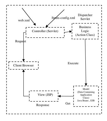
Figure 1 Component in the Struts Architecture
