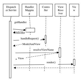
Figure 5: Sequence flow of application in the spring framework.
