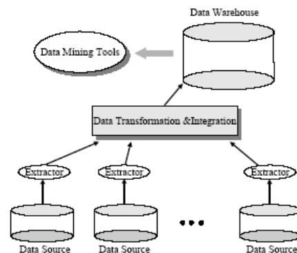
Figure 1. A data warehouse architecture
