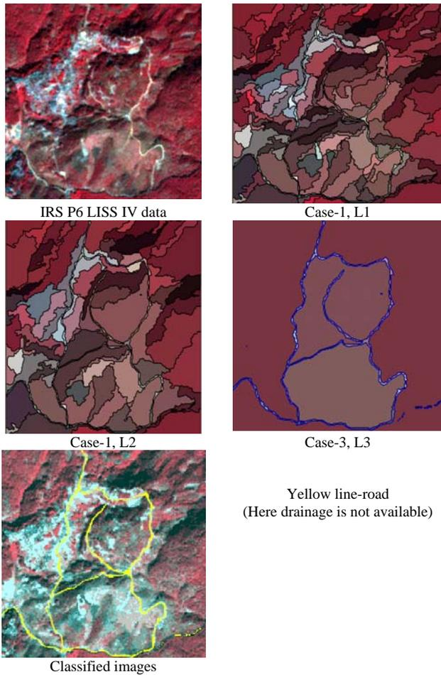
Figure 2. Segmentation and classification for IRS P6 LISS IV images
