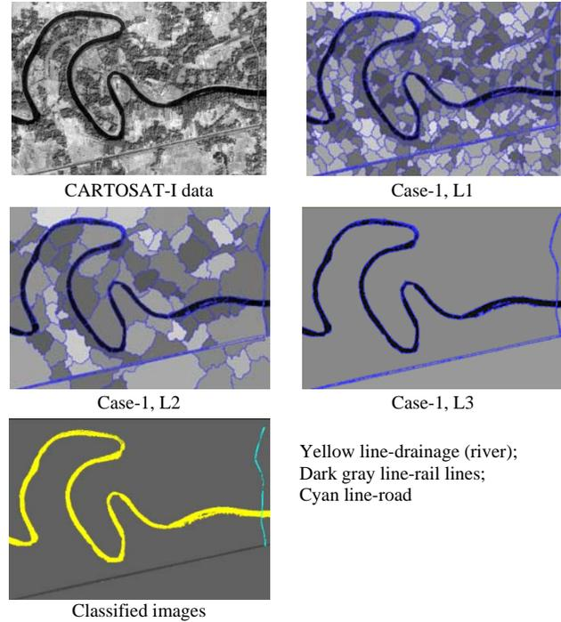
Figure 1. Segmentation and classification for CARTOSAT-I images
