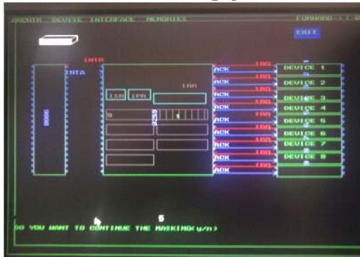
fig.sim.16.Priority resolving when multiple I/O devices are connected to the system.It is showing Device 5 is masked and running under fixed priority mode.
