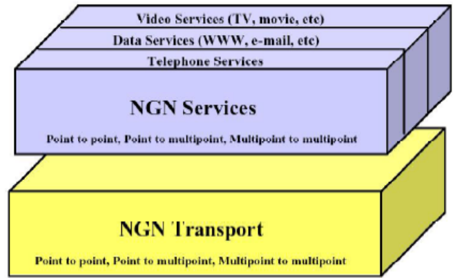
Figure 2. Separation of functional planes
