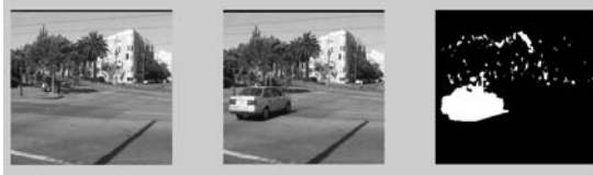
Figure 6. Background subtraction for the adaptive video without fuzzy interference
