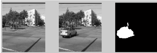
Figure 7. Background subtraction for the adaptive video with fuzzy interference
